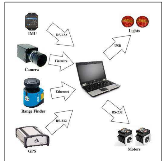
FIGURE 4 : COMMUNICATION PROTOCOLS BETWEEN THE COMPUTER AND THE SENSORS
